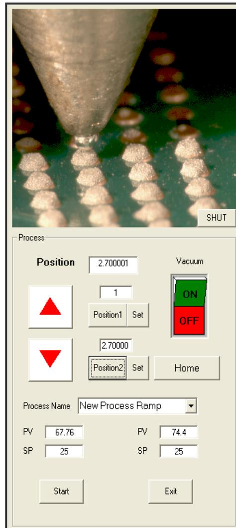
**Figure 5:** Front panel of the computer control interface
