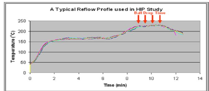
**Figure 6:** One of the profiles used in the HIP study. Temperature reproducibility is within 5-6°C, which is comparable with a typical reflow oven.
