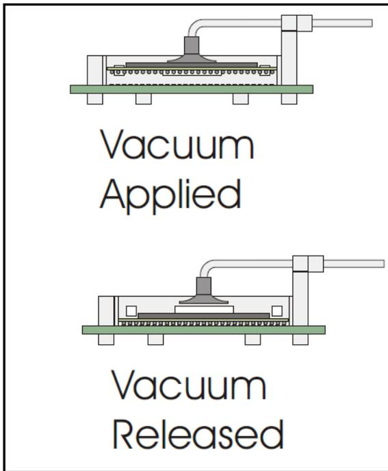
**Figure 1:** A view of the HIP test set-up using a BGA Rework station
