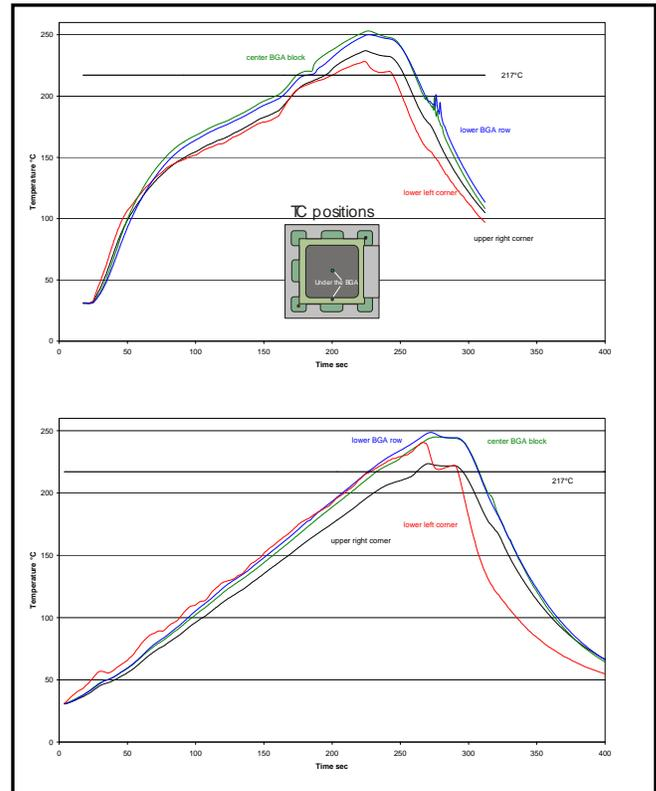
**Figure 2:** High Soak and Straight ramp reflow profiles
