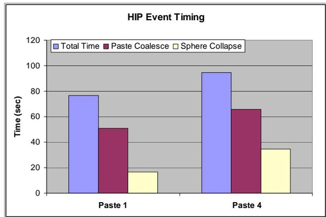
**Figure 8:** Comparison of coalesce and sphere collapse times.
