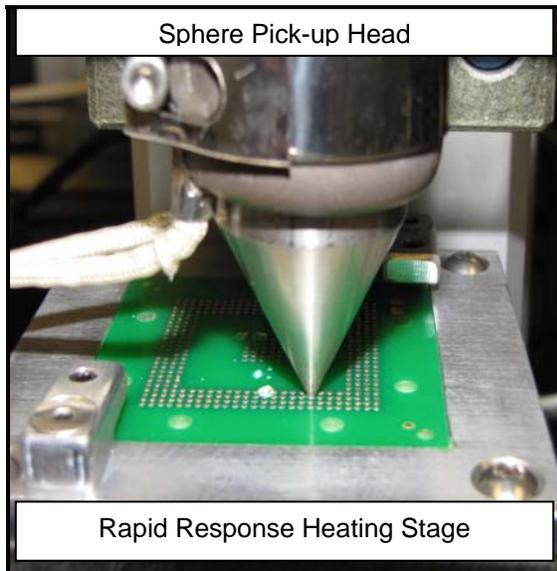
**Figure 4:** A view of the HIP test apparatus
