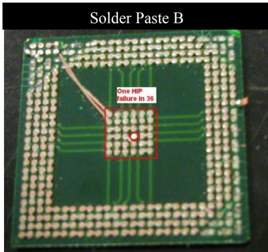
Figure 3d: PBGA component showing 1 HIP defect
