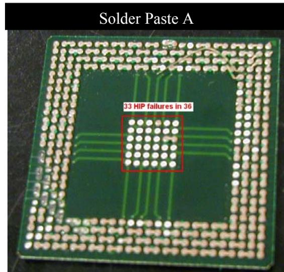
**Figure 3a:** PBGA component showing 33 HIP defects
