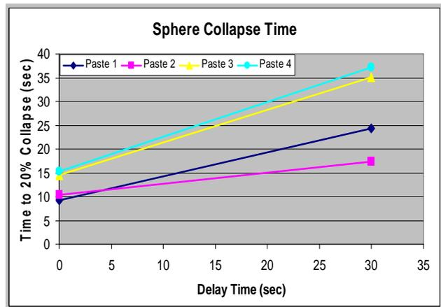
**Figure 10:** Dependence of the time for 20% sphere collapse on the delay in ball placement.
