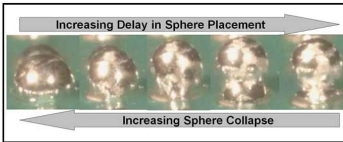
**Figure 9:** Collapse of solder sphere as a function of sphere placement time (time delay in placement in creating HIP defect)
