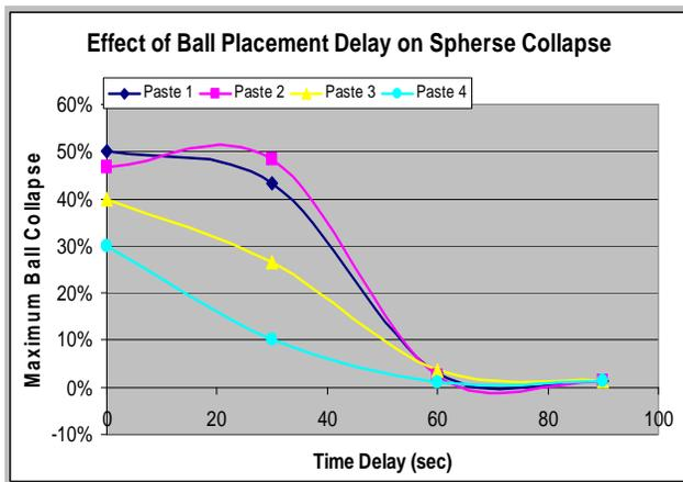
**Figure 8:** Dependence of sphere collapse on the time delay between the paste coalescence and the ball placement.
