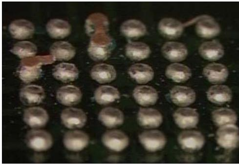
Figure 3b: PBGA component pruned from the test vehicle
