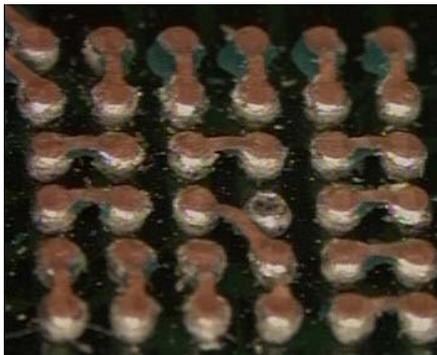
Figure 3e: PBGA component pruned from the test vehicle
