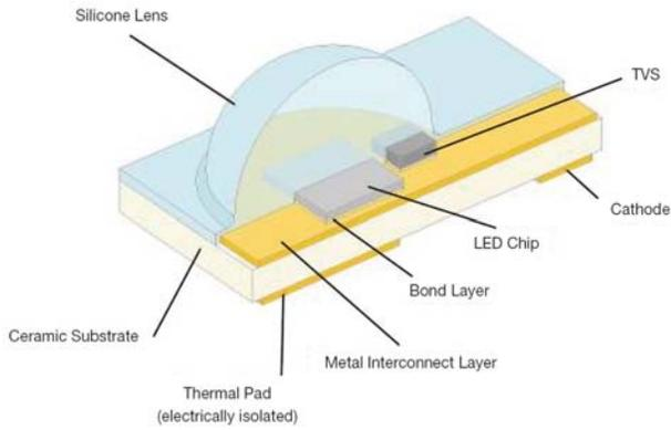
**Figure 2.** Cross section of LUXEON Rebel package
