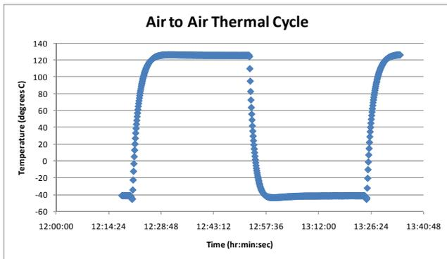
**Figure 7:** Thermal cycles as measured in the Thermotron environmental chamber
