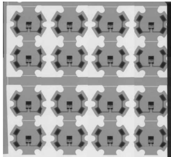
**Figure 3.** MCPCB Test Vehicle used for the study
