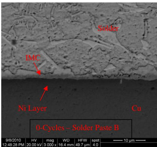
**Figure 9.** SEM micrographs of solder joints on MCPCB A for Solder Paste A and Solder Paste B
