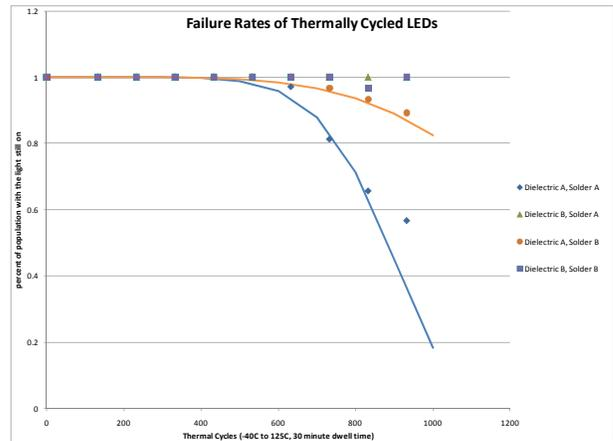
**Figure 8:** Failure rate vs. number of thermal cycles of combinations of MCPCB dielectrics and solders
