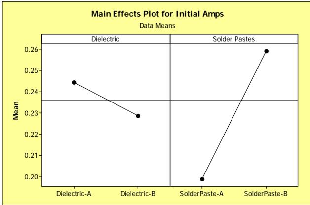
**Figure 6.** Initial Amperage for different solder pastes and board dielectrics
