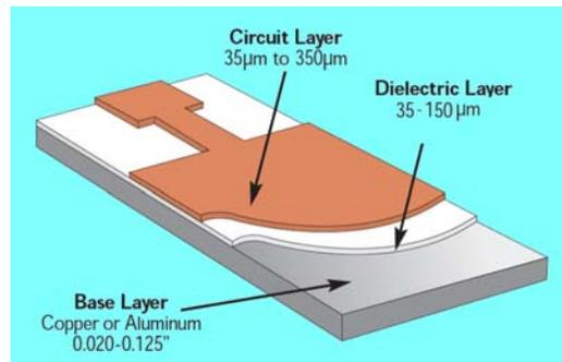
**Figure 4.** Cross section of a typical MCPCB
