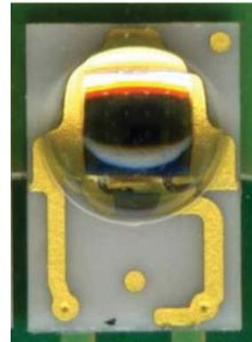
Figure 1. Image of InGaN LED package
