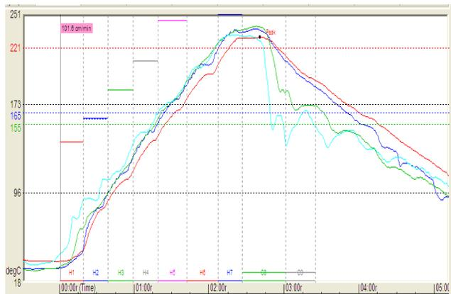
**Figure 4.** Profile 3: Straight Ramp 1.35°C/s 230°C Peak 45s TAL
