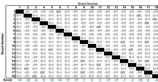
Figure 13. Visual inspection results—comparison of 0.15 mm pads/0.15 mm spacing.
