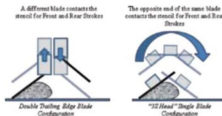
Figure 1. Comparison of the YGP 3S (Swing Single Squeegee) to the standard double trailing edge blade configuration.
