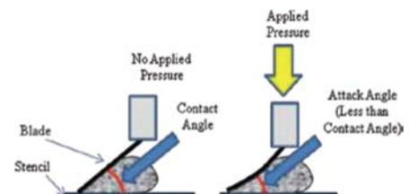
Figure 2. Contact angle vs. attack angle.
