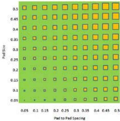
Figure 3: Test board design (all units in mm).
