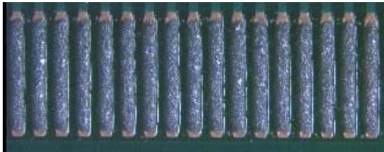
Print speed = 1 in./sec (25.4mm/sec) Squeegee pressure = 1 lb/linear in. (0.18 Kg/cm)
