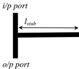
**Fig. 1 :** Structure of microstrip T-resonator
