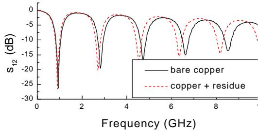
Fig. 6 : T resonator response for bare copper boards and boards printed with flux
