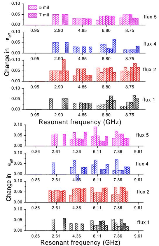
**Fig. 9 :** Comparison of change in  $e_{eff}$  caused by solder pastes measured on (a) T1 and (b) T2 resonators
