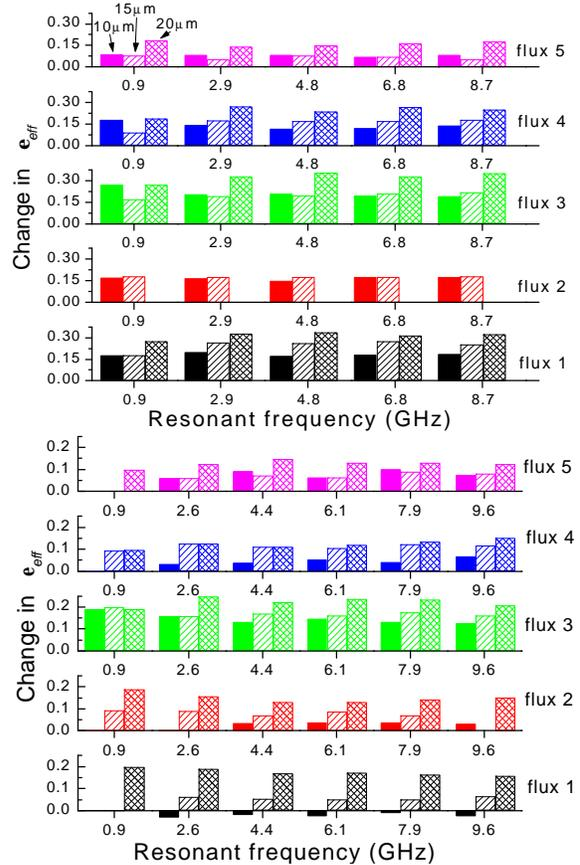
Fig. 7 : Comparison of change in  $\epsilon_{eff}$  caused by fluxes measured on (a) T1 and (b) T2 resonators
