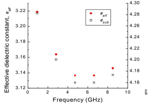
Fig. 5 : Effective dielectric constant,  $e_{eff}$  and substrate dielectric constant,  $e_{sub}$ , vs. frequency for FR4
