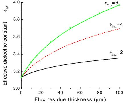
Fig. 4: Effective dielectric constant vs. residue layer
