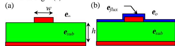
**Fig. 3 :** (a) Microstrip structure, (b) with flux residue
