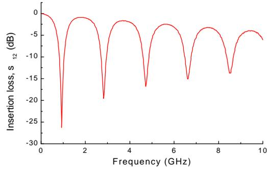
**Fig. 2 :** Typical T-resonator response
