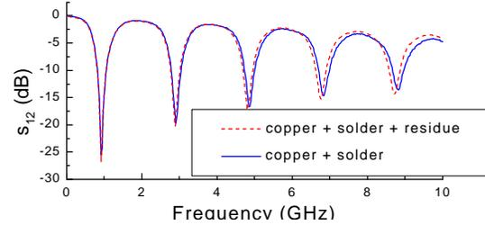
**Fig. 8 :** T resonator response illustrating effects due to flux residue
