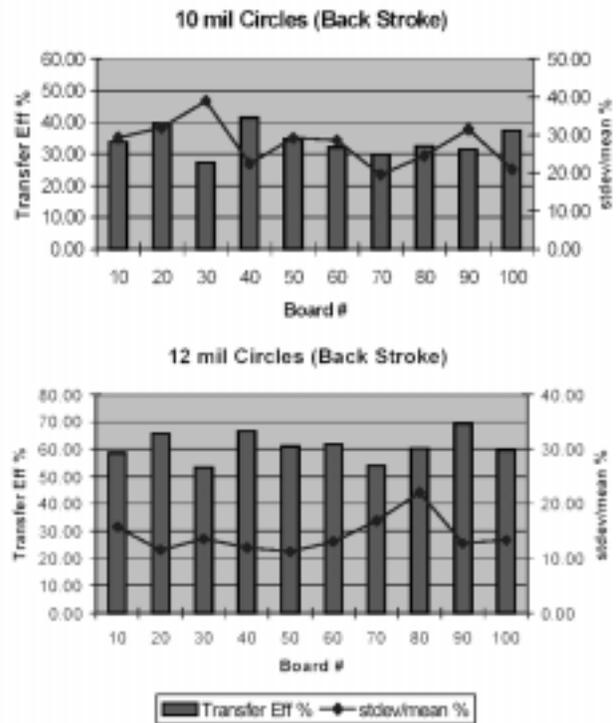
**Figure 10: Effect of boards printed without wiping.**
