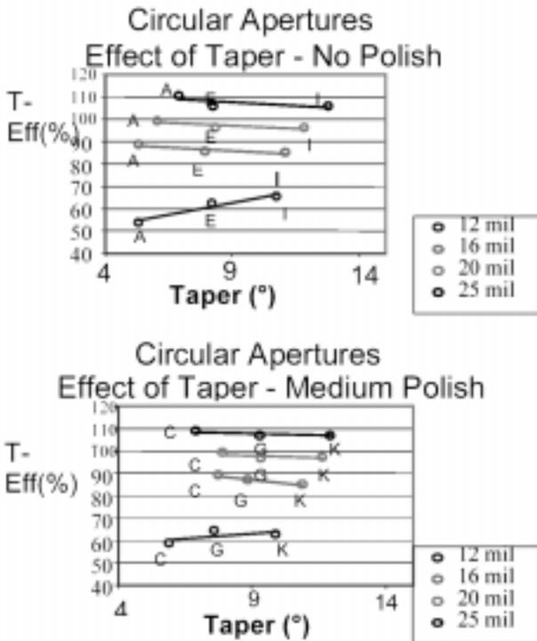
**Figure 9: Effect of taper on transfer efficiency.**
