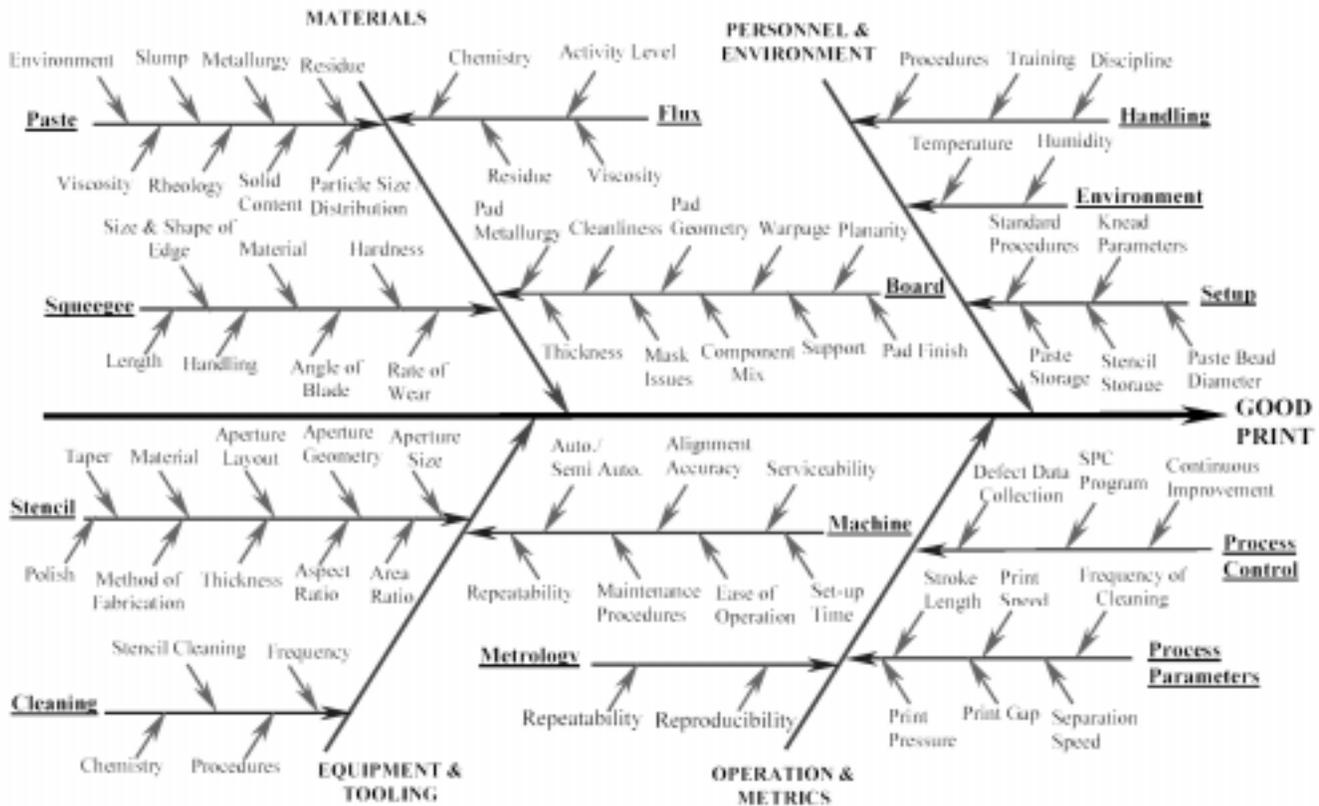
Figure 1: Fishbone-stencil printing factors.
