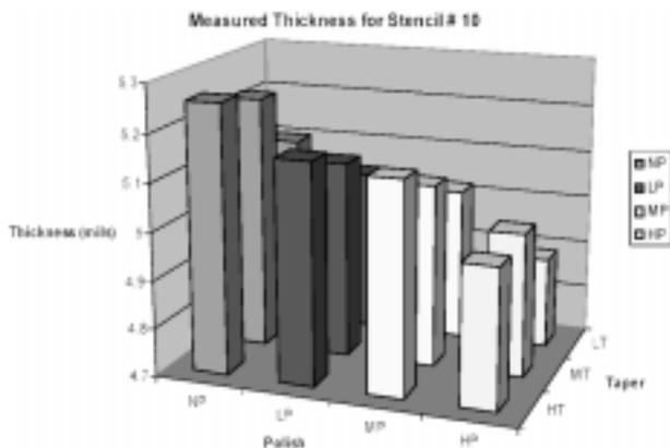
Figure 7: Thickness variation with increased electropolish.
