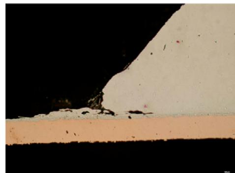
Figure C5. The fatigue crack emerging at the outer edge of the soldered joint
