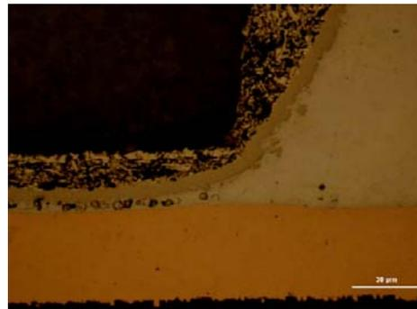
Figure B6. Higher magnification micrograph of a fuller SAC-X 0307 solder joint 0805 chip resistor showing increased grain definition and de-lineation
