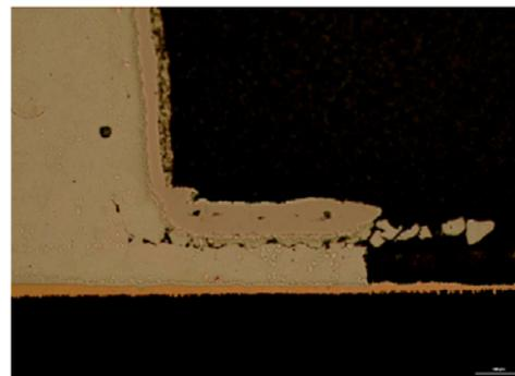
Figure C10. A higher magnification image of the thermal fatigue cracks
