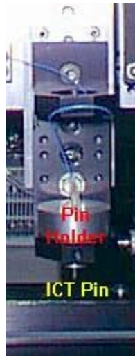
Figure 1. ICT probe holder for Camalot 3800 Dispensing System pin testing.
