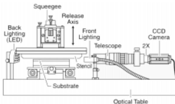
**Figure 1: Schematic of real time print dynamics visualization platform.**
