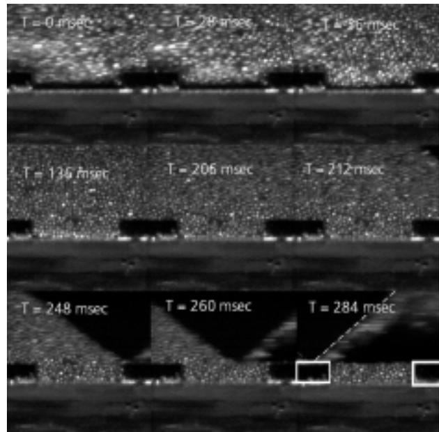
Figure 14: Sequence of paste flowing into a 0.025" wide aperture.
