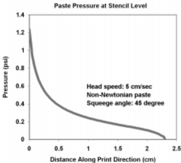
Figure 13: Pressure distribution at stencil level.
