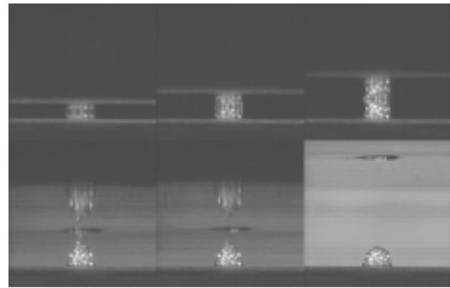
Figure 5: Sequence of paste releases from 10 mil diameter round aperture, electroformed 6 mil thick stencil with Paste C.
