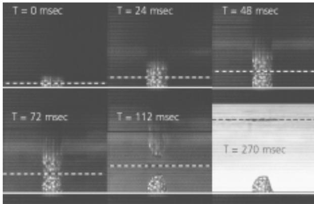
Figure 3: Sequence of real time paste releases from 10 mil diameter round aperture, laser cut 6 mil thick stencil with Paste C.
