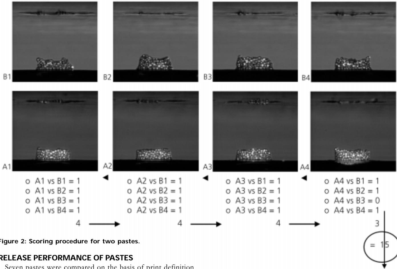
Figure 2: Scoring procedure for two pastes.
