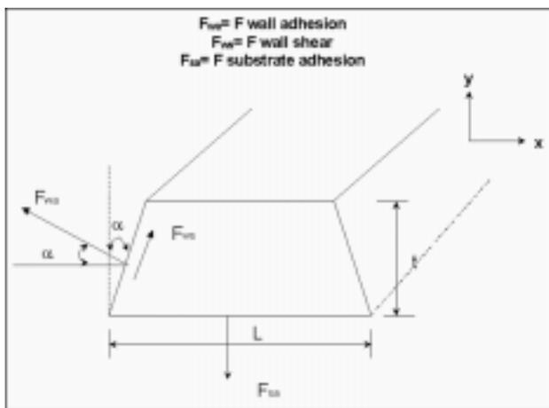
Figure 8: Nomenclature for paste release model.
