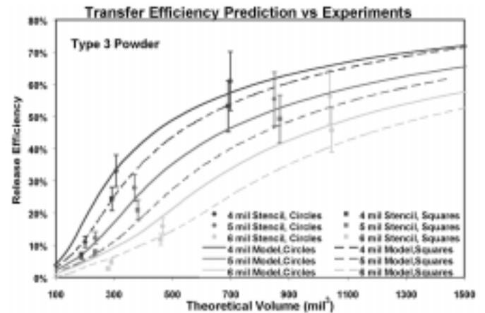
Figure 10: Release efficiency predictions and experiments for Type 3 paste, various stencil thickness and aperture geometry.
