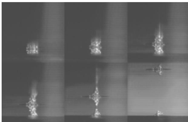
Figure 4: Sequence of real time paste releases from 10 mil diameter round aperture, laser cut 6 mil thick stencil Paste D.
