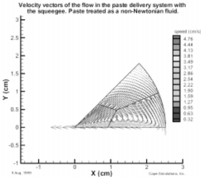
Figure 12: Paste flow simulation for a squeegee system.
