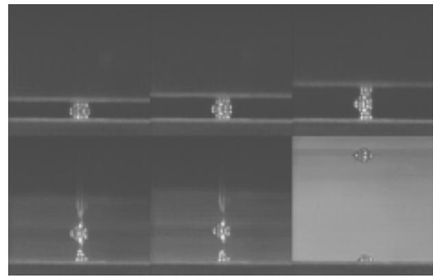
Figure 6: Sequence of paste releases from 10 mil round aperture, chemical etched 6 mil thick stencil with Paste C.
