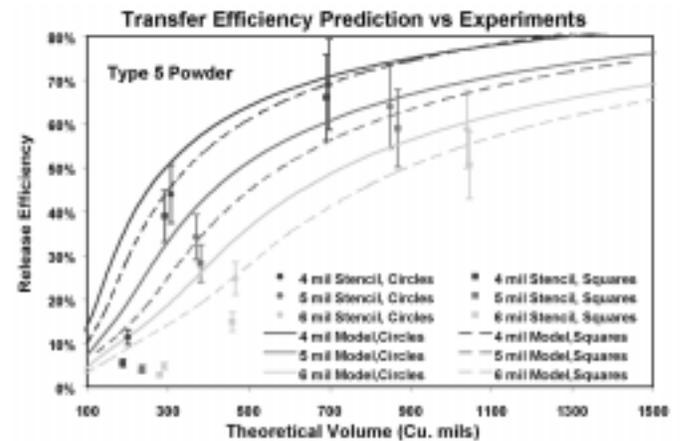
Figure 11: Release efficiency predictions and experiments for Type 5 paste, various stencil thickness and aperture geometry.
