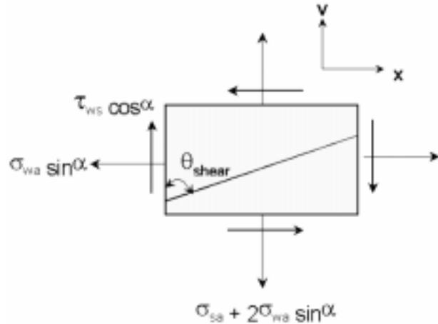
Figure 9: Normal and shear stress diagram for an elemental volume of paste.
