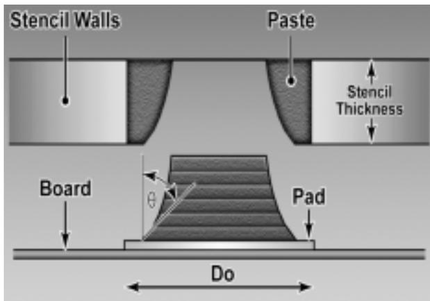
Figure 7: Schematic of paste release mechanism.
