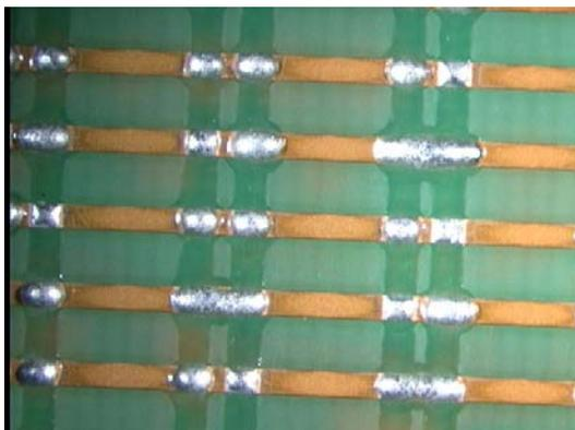
**Figure 2 .** Wetting test cross-print post reflow
